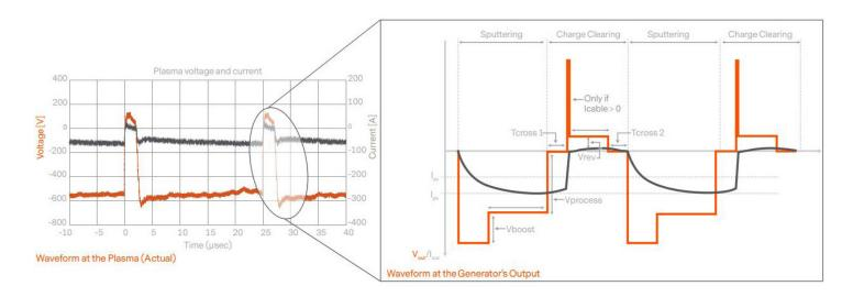
A patented boost circuit on the leading edge of the sputtering waveform accelerates delivery of power to the process compared to a sine wave generator. The reverse portion of the waveform maximizes control, allowing more definitive charge clearing during reverse cycle.
