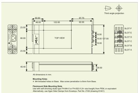
Note: XCE, XVE, XFA, XFB, XFC, XFN dimensions L=268mm
