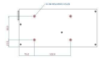
Mounting Holes: 4 x M4 threaded PEMs on Base. Max Screw Penetration is 2mm from Base. 2 x M3 threaded PEMs on Each Side. Max Screw Penetration is 2mm from Side.
