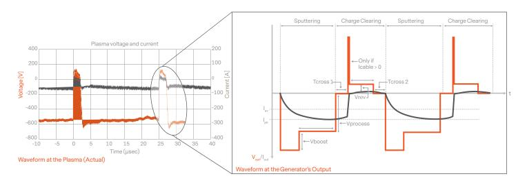
Use as a single-magnetron sputtering supply or as a bias supply.
